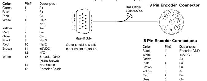
(Shield should not be connected at this connector)
